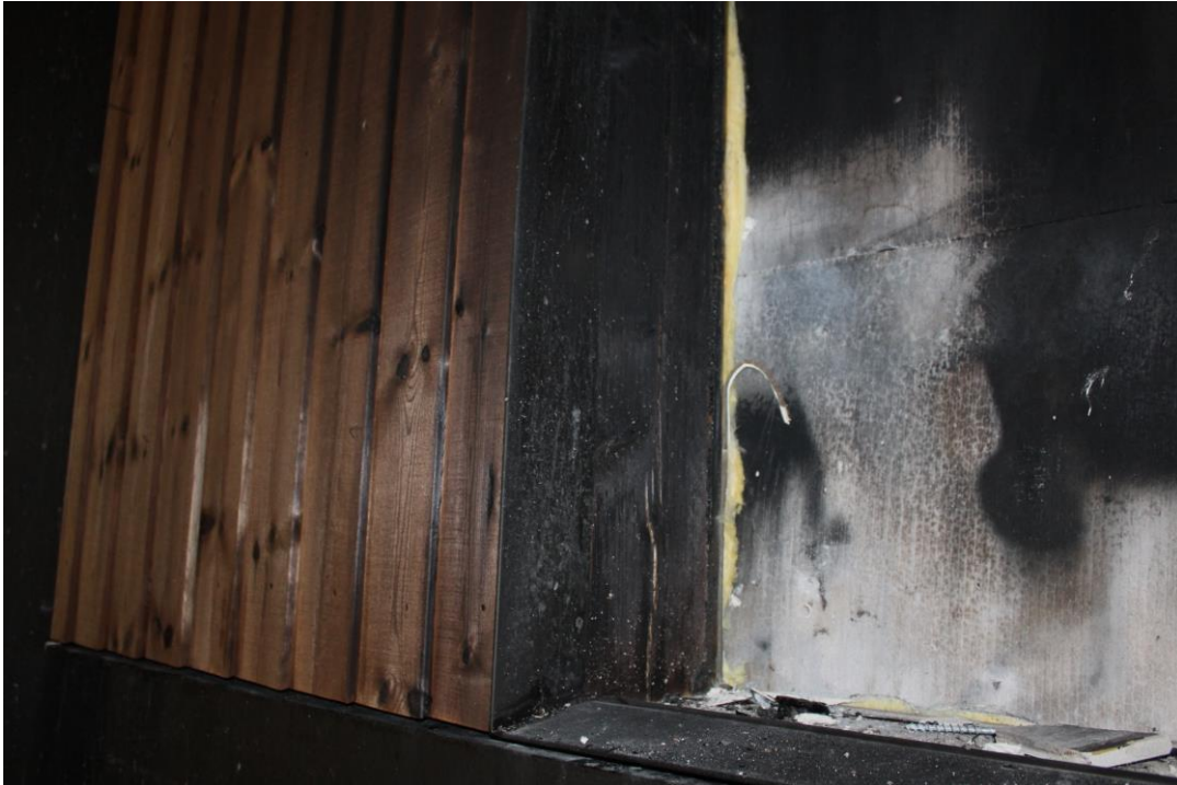
Photo No. 27 Test specimen after the test. Detailed photo of 2. Floor left bottom corner.
