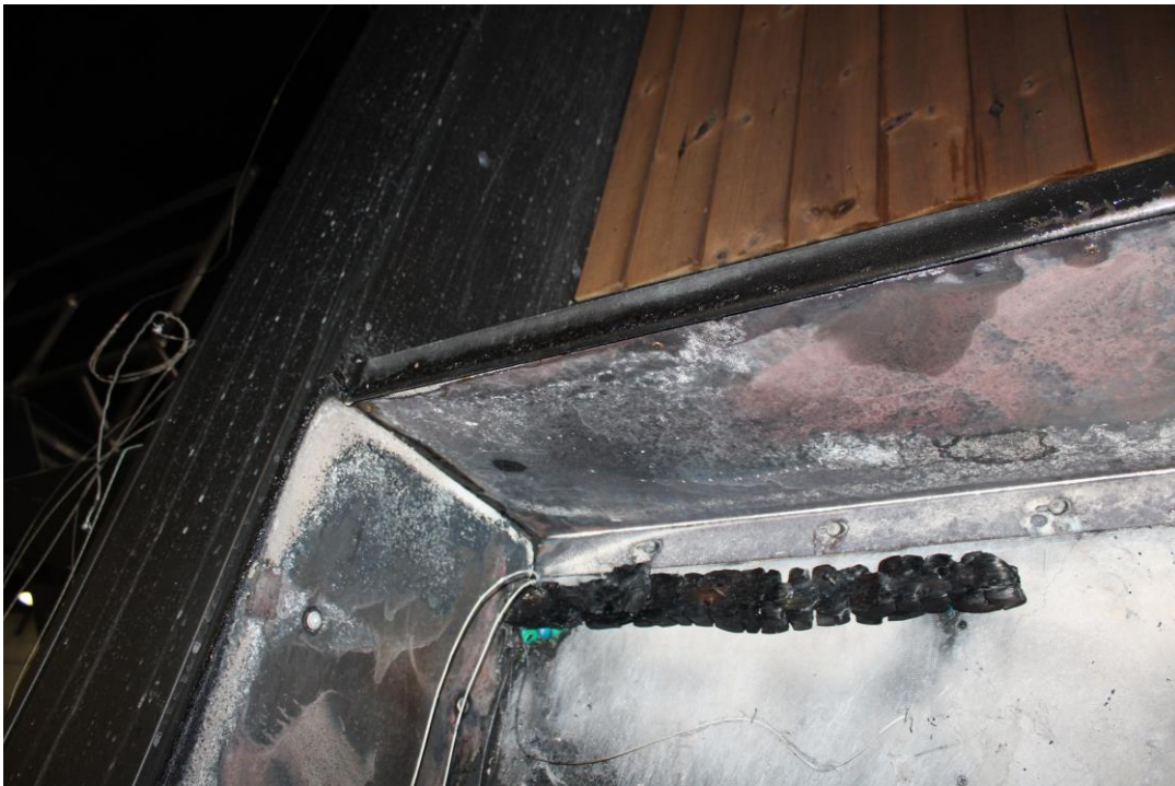
Photo No. 26 Test specimen after the test. Detailed photo of 1. Floor left top corner.
