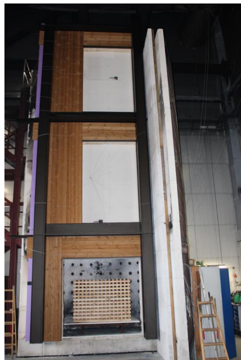
Photo No. 9 Vertical and horizontal cladding have been mounted.
