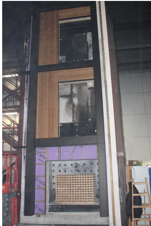
Photo No. 9 Vertical and horizontal cladding have been mounted.
