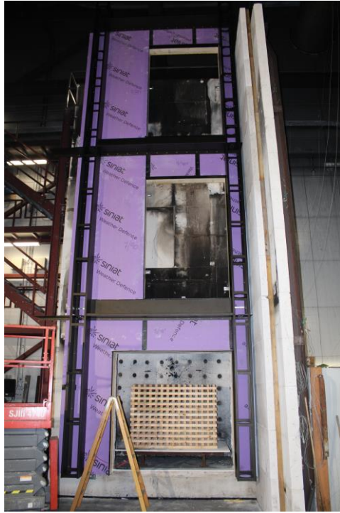
Photo No. 7 Vertical steel projector added to the prefabricated elements.
