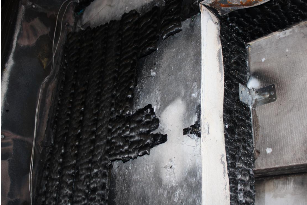
Photo No. 23 Test specimen after the test. Detailed photo of the façade
